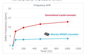
Murata MEMS exhibits stable frequency stability even under harsh environment by eliminating organic material inside the package.
