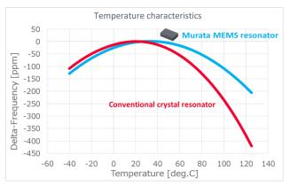
Good temperature characteristics are realized by optimizing device structure and design.
